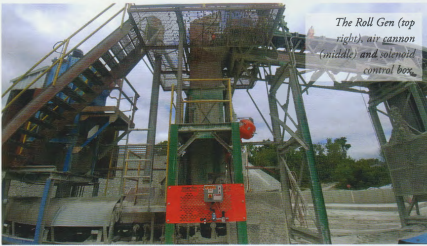
The 70-L Hurricane Air Cannon features a fan jet nozzle for wide coverage.
