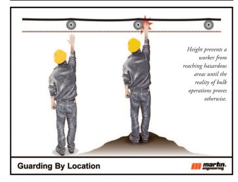
workers or walkways. Guarding by location is the assumption that when hazards, such as moving conveyor belts, are positioned beyond the normal reach of a worker they don't require a guard. Yet they can still present a serious hazard.
