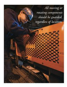
points, shear points and moving or rotating components should be guarded, regardless of location or access.
