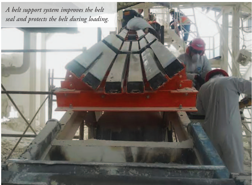
External wear liner and dual self-adjusting seal with belt support.
