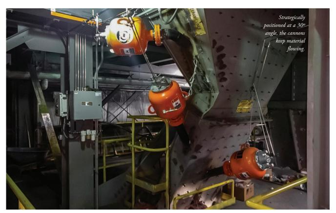
the vessel surface. Instead, the fact that the polymer lining was bolted to the vessel caused it to muffle the vibration of the units, limiting the force to only the impact zone and not much farther.
