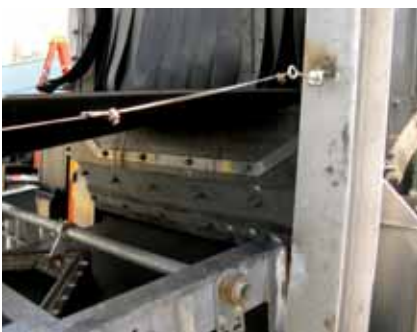
Discharge area with seal between carrying and return sides of the belt.
