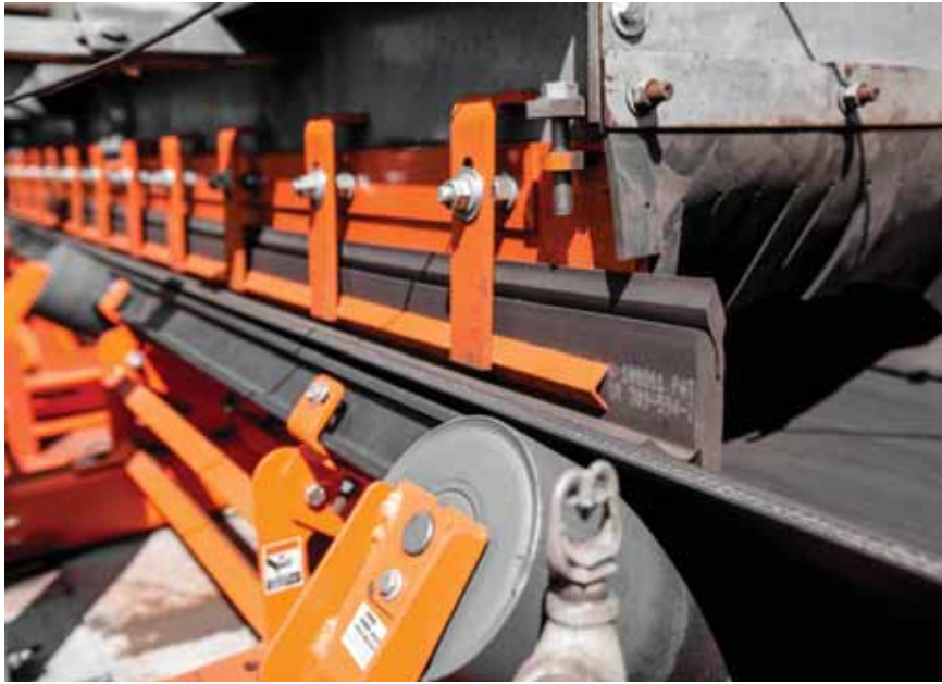
Settling zone with wear liner, apron seal & dust curtain.
