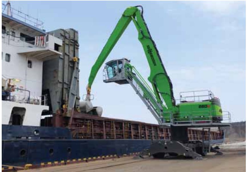
SENNEBOGEN 860 E-Series with Green Hybrid Energy Recovery and Skylift cab elevation
