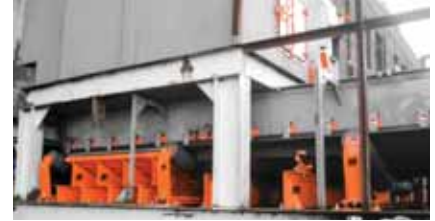
Support cradles help flatten the belt path for effective sealing.
