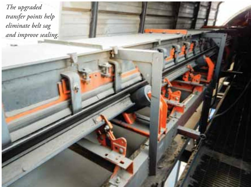
*The upgraded transfer points help eliminate belt sag and improve sealing.*
