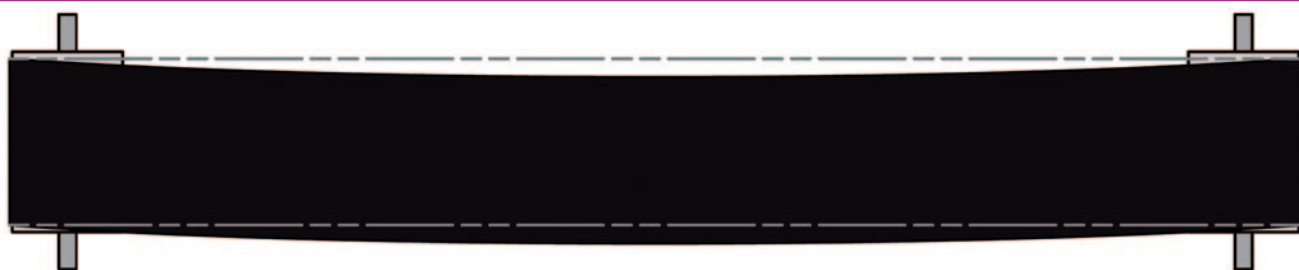
Figure 1 – Camber can happen in the manufacturing process, and belts should be inspected prior to installation (© 2022 Martin Engineering).
