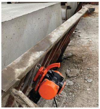
Responding to the precast operators who have static forms or need units readily transferred from one form to another, Martin Engineering designed an optional ductile iron wedge and sturdy curved handle for MHF-1500 Brushless Concrete Vibrator portability and versatility.
