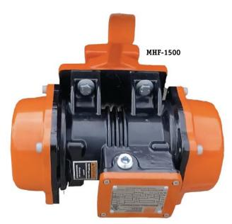
washing. The casing can be opened for easy maintenance in-house. By removing the weight covers, operators can adjust the vibratory unbalance to the required force needed for the application. Each MHF-1500 features oversized and permanently lubricated roller bearings contained in sealed ductile iron housings, adding to the unit's long service life. — Martin Engineering, Neponset, Ill., 309/852-2384 or 800/544-2947; www.martin-eng.com
