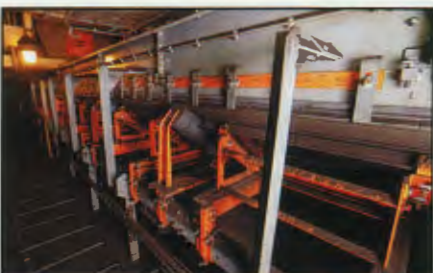
Inspection doors and track-mounted components facilitate maintenance for extended equipment life.
