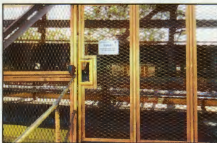
A gate to a conveyor walkway, controlled with an RFID sensor.
