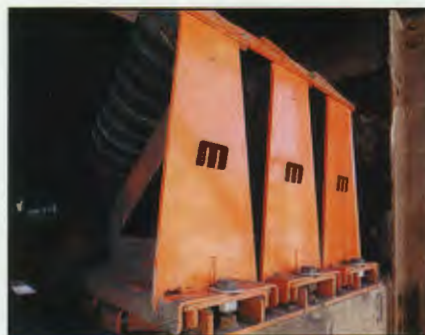
Track-mounted idlers allow easy access for quickly swapping out seized rollers.
