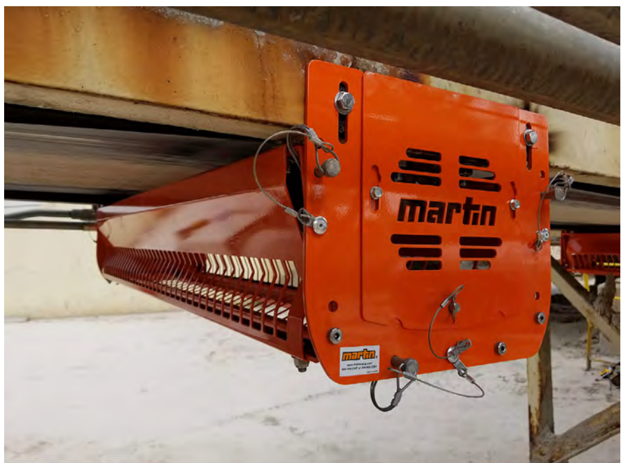
Return roller guards ensure detached rollers don't pose a hazard to workers or harm the system.
