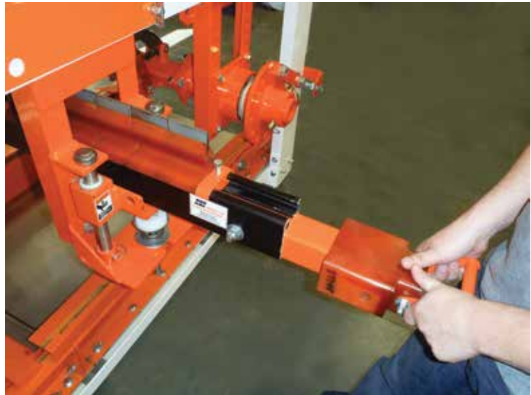
This slide-out belt cleaner is engineered to be accessed safely and replaced by a single worker.
