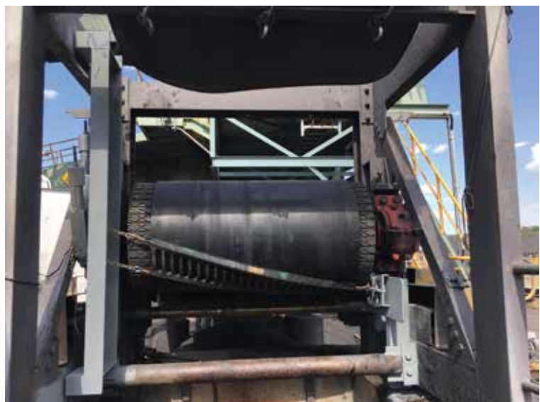
The unique belt cleaner forms a 3-D curve beneath the discharge that conforms to the pulley’s shape.
