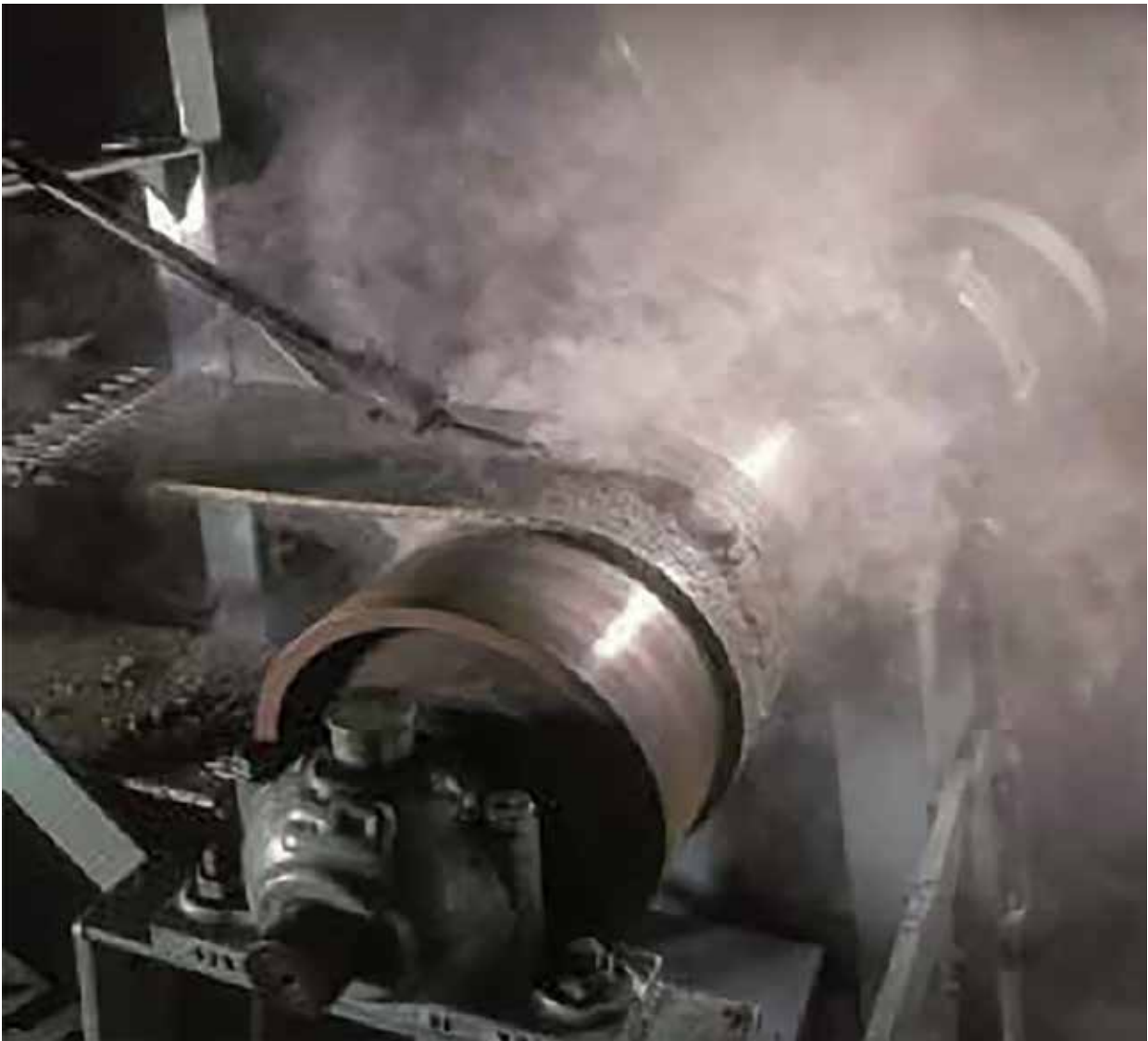
Friction heat between rolling components can be extreme enough to light both the material and belt.
