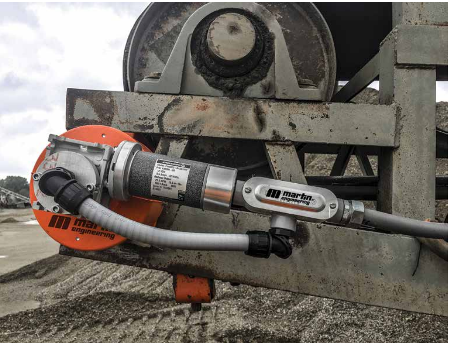
Automatic tensioner maintains optimum cleaning pressure without operator intervention.
