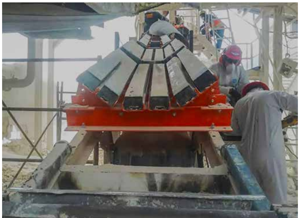
Figure 8: Impact cradles minimise belt damage and improve edge sealing.
