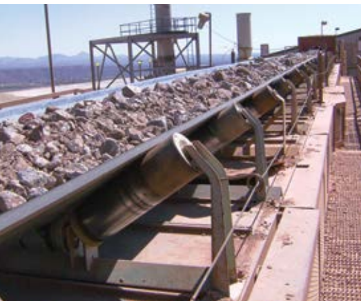
Conveyor with proper loading and tracking.
