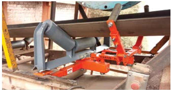
Modern belt training devices detect slight variations in the belt path and correct it immediately to retain production efficiency.
