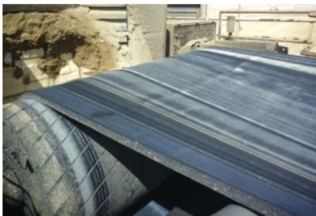
Figure 2 — Grooves can be created along the entire length of the belt under the skirt.
