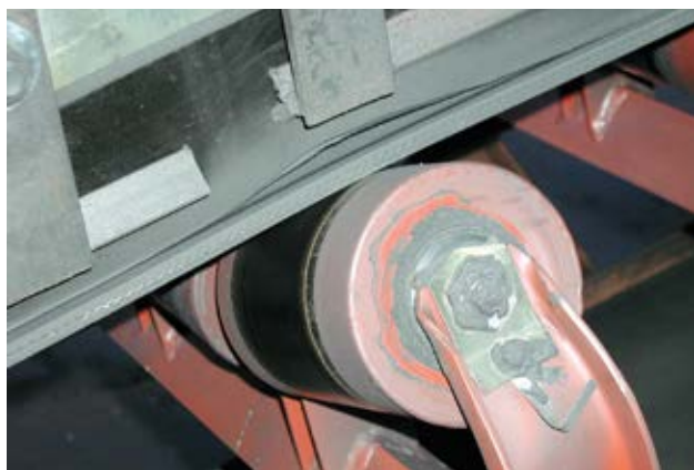
Figure 1 — Scalping occurs when trapped material forms a high-pressure area between the roller and the skirt.
