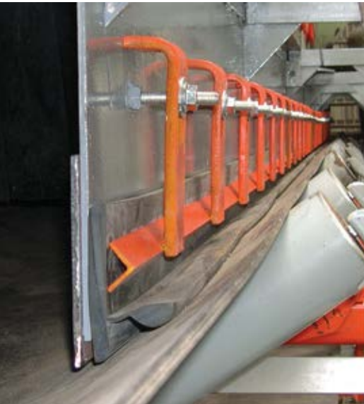
Figure 7 – The external configuration redesigns the chute for more effective sealing.
