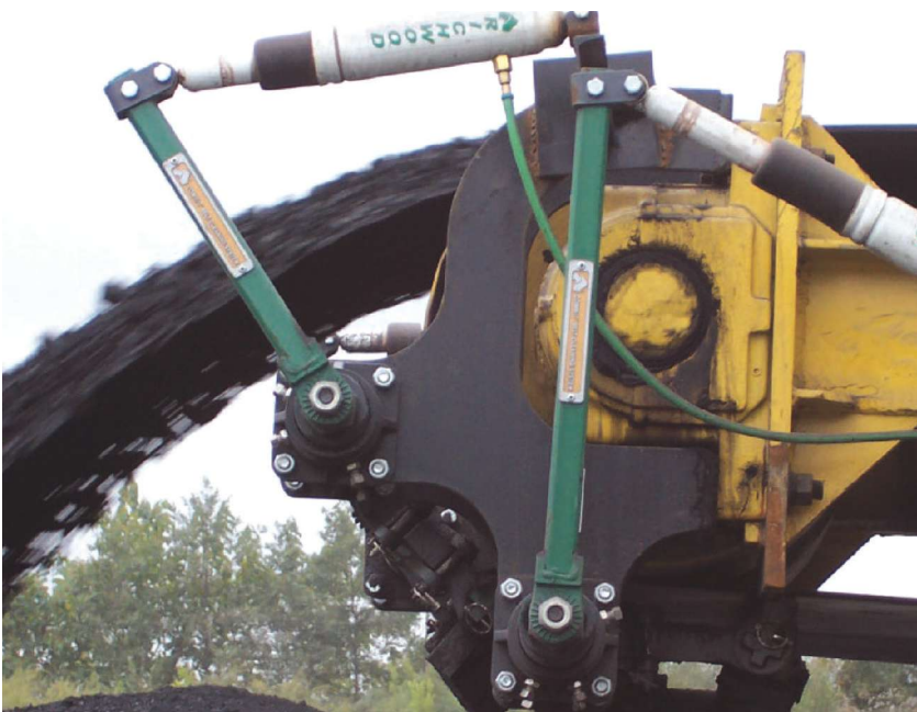
With a self-adjusting tension system, Richwood's cleaners can be located in primary or secondary positions.
