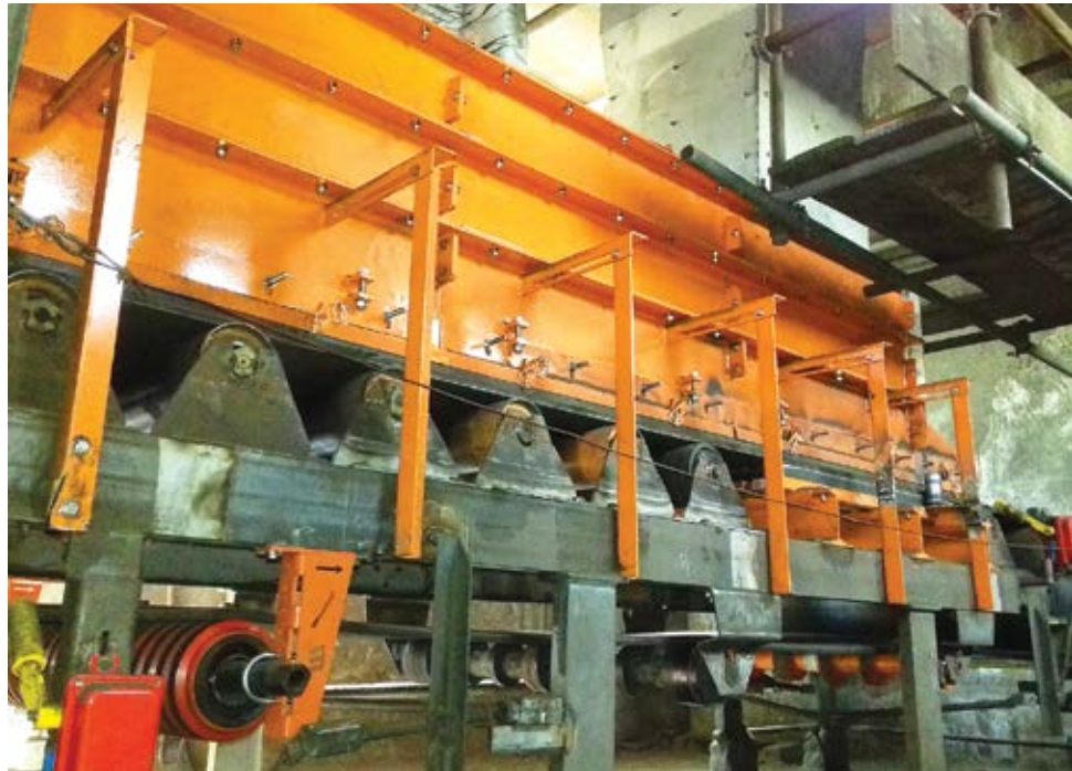
Martin Engineering's modular transfer kit installs easily and facilitates future upgrades.
