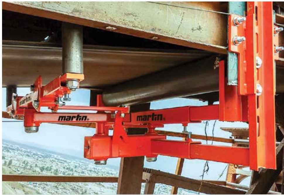
A multi-pivot trainer manages the load-carrying run of the conveyor. (Photo: Martin Engineering)
