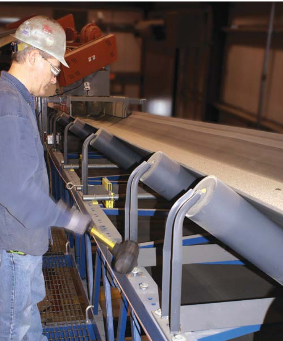
“Knocking” an idler will cause the tracking to change, but it’s not a reliable means of solving alignment issues. (Photo: Martin Engineering)
