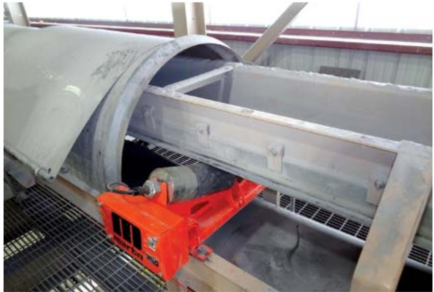
A single Roll Generator has enough power output to run a variety of accessories.
