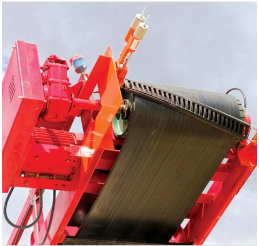
The CleanScrape forms a 3-D curve beneath the discharge that conforms to the pulley’s shape. (Photo: Martin Engineering)
