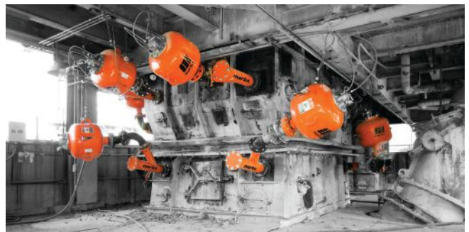
The old 150-liter cannons with fixed pipe assemblies.
