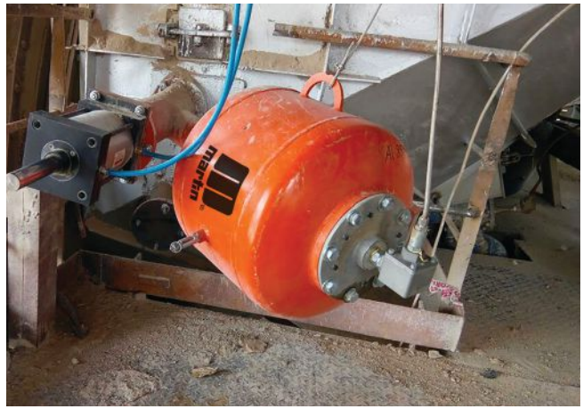
A single cannon to address a clog point, with a retractable nozzle to extend the equipment life.
