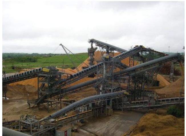
A wide range of alternative fuels like bagasse pictured here are used as fuel in the production of cement.
