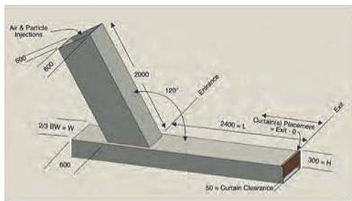
Figure 4: Standard conveyor
