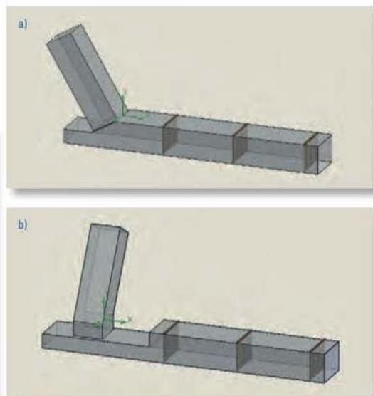
Figure 9: a) preferred inline transfer new construction; b) preferred angle or retrofit transfer
