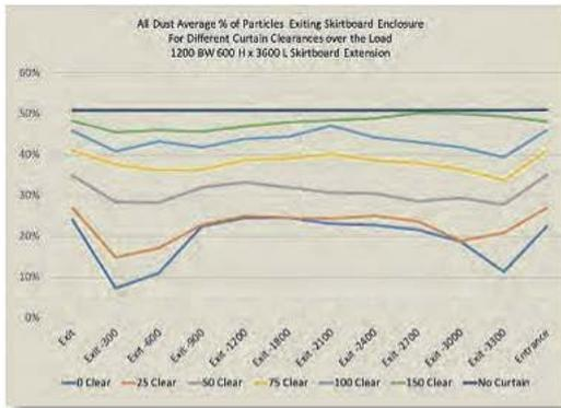
Figure 12: Curtain clearance above load vs dust emissions
