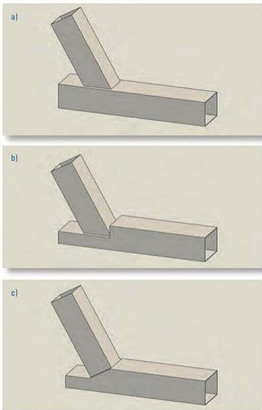
Figure 5: a) standard chute configuration; b) retrofit; c) mitered
