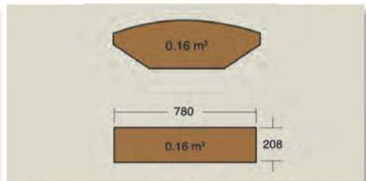
Figure 3: Cross-sectional area per meter
