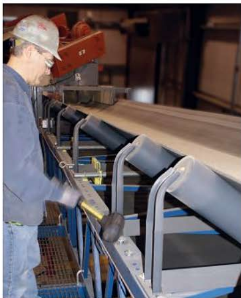
Figure 1: "Knocking" an idler with a mallet to change its position
