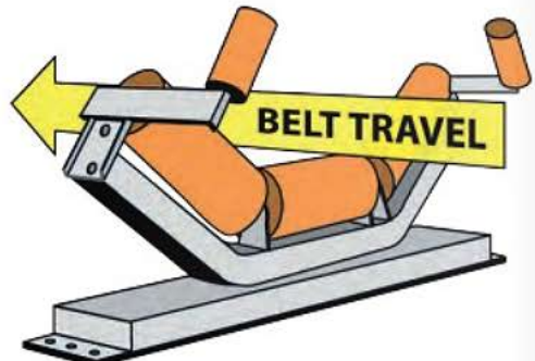
Figure 2: Tracking idler (all photos and graphics by Martin Engineering Company, Neposet, USA)
