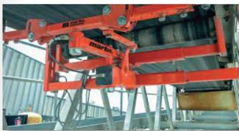
Figure 6: The return side Martin Tracker lifts the belt slightly for appropriate contact
