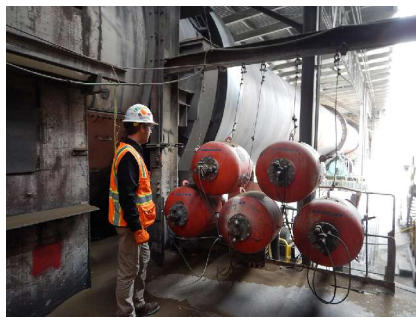
Valves face outward for convenient maintenance, requiring no tank removal to service them.
