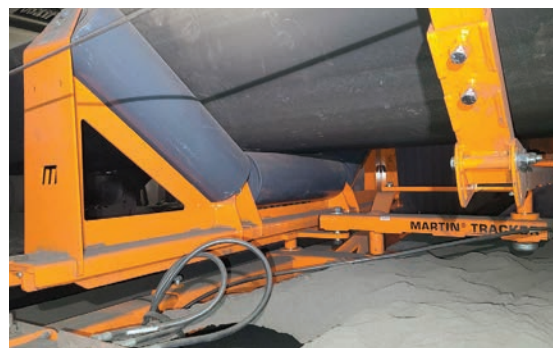
The pivoting idler assembly rotates in the opposite direction of the mistracking belt. CREDIT: MARTIN ENGINEERING
