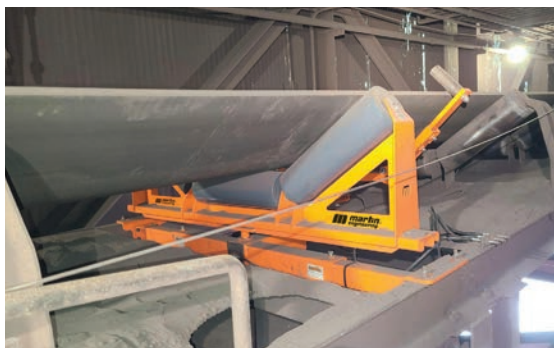
The torsion rollers ride smoothly on the belt edge, detecting slight variations in the belt path. CREDIT: MARTIN ENGINEERING
