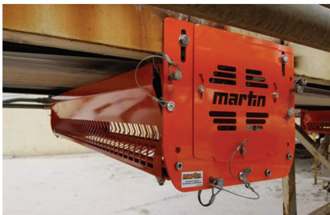
Return roller guards ensure detached rollers do not pose a hazard to workers or harm the system. CREDIT: MARTIN ENGINEERING
