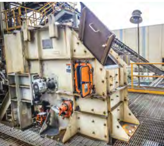
Inspection doors and track-mounted components facilitate maintenance for extended equipment life.
