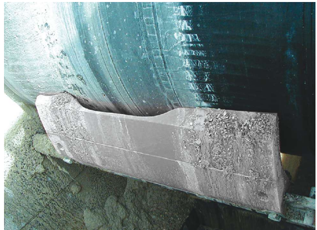
Figure 2—As the center of the blade wears unevenly, the outer edges create an effect called a 'smiley face' or 'mooning.'
