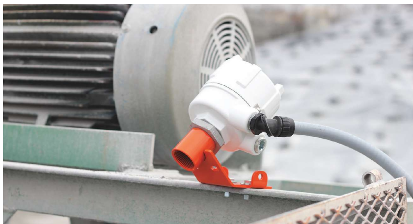
Figure 6—Sensors are used to back the blade away during stoppages or when running empty.
