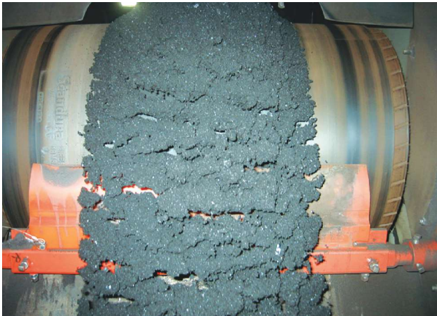
Figure 1—When the blade is wider than the material flow, its center may wear quicker than the outer edges.
