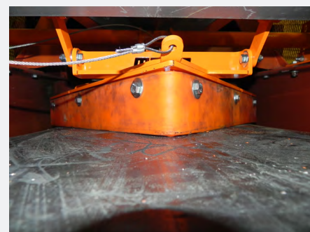
THE V-PLOW HD HUB MOUNTS CAN BE WELDED OR BOLTED TO THE HANGER BARS. © 2021 MARTIN ENGINEERING
