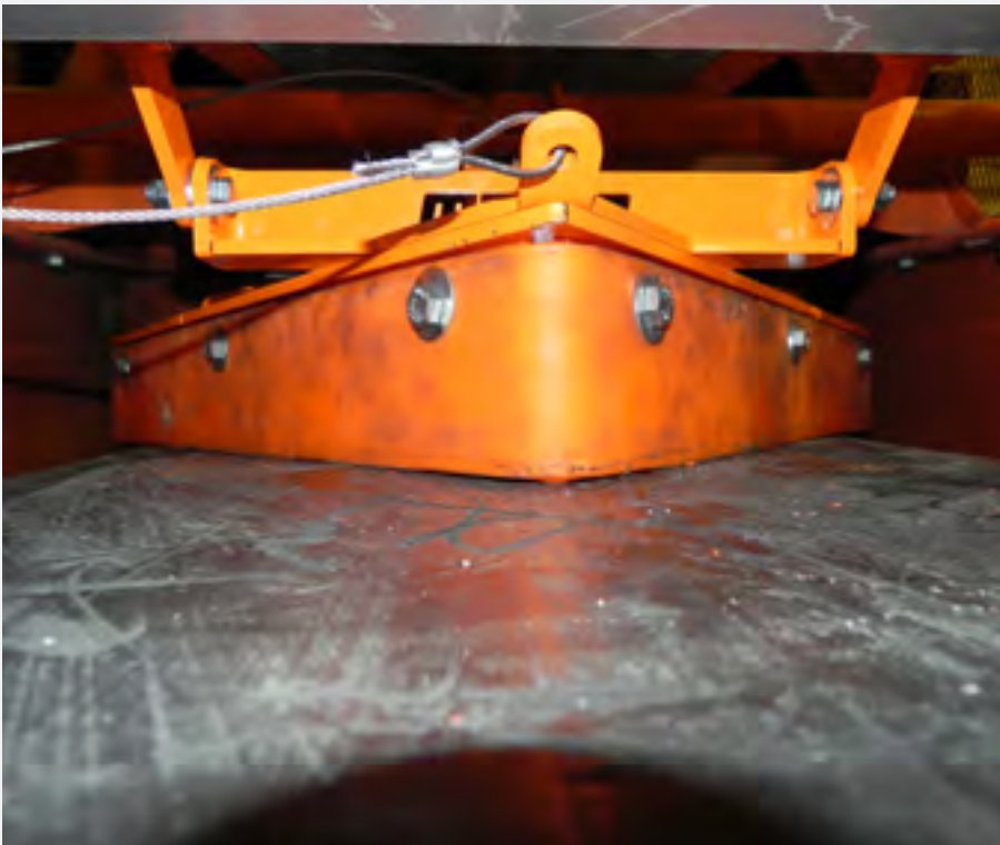
THE V-PLOW HD HUB MOUNTS CAN BE WELDED OR BOLTED TO THE HANGER BARS
