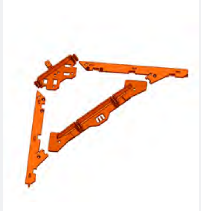
THE MODULAR REDESIGN IS EASIER AND SAFER TO TRANSPORT, REQUIRING MINIMAL ASSEMBLY ON-SITE
