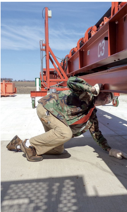
TAKING A SHORTCUT BY CROSSING OVER OR UNDER A CONVEYOR CAN LEAD TO INJURY © MARTIN ENGINEERING 2021
