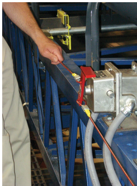
SAFETY EQUIPMENT SUCH AS PULL STOPS AND EMERGENCY SWITCHES ARE VITAL TO CONVEYOR SAFETY © MARTIN ENGINEERING 2021
