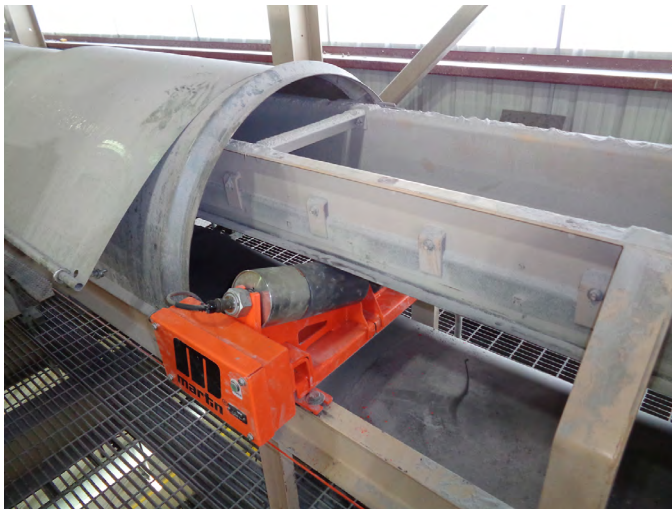
A SINGLE ROLL GENERATOR HAS ENOUGH POWER OUTPUT TO RUN A VARIETY OF ACCESSORIES © MARTIN ENGINEERING 2022
