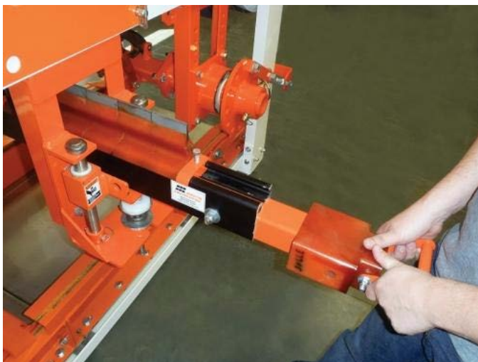
THIS MARTIN SQC2S STS SECONDARY CLEANER ALLOWS FOR SAFE EXTERNAL MAINTENANCE BY A SINGLE WORKER
