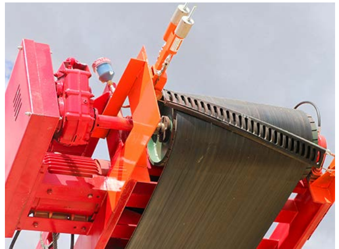
THE CLEANSCAPE® FORMS A 3-D CURVE BENEATH THE DISCHARGE THAT CONFORMS TO THE PULLEY'S SHAPE (ALL IMAGES © MARTIN ENGINEERING 2023)
