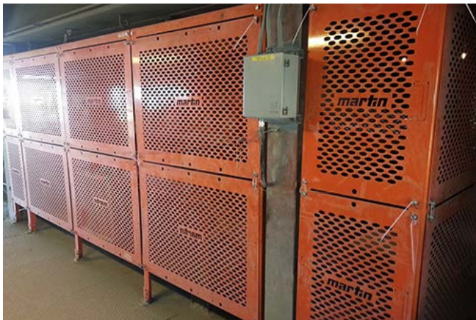
MARTIN® GUARDING IS DESIGNED TO PROTECT WORKERS FROM REACH-IN INJURIES IN UNAUTHORISED AREAS
