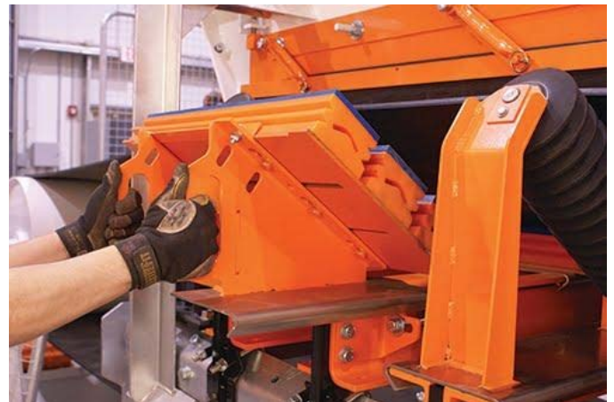
THE TRACK-MOUNTED MARTIN® SLIDER CRADLE CAN BE SERVICED QUICKLY AND SAFELY, WITH NO REACH-IN MAINTENANCE.
