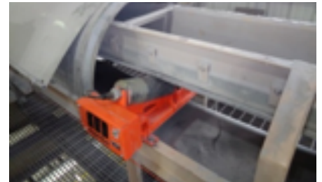
THE OD OF THE GENERATOR MATCHES THAT OF THE ROLL, BUT PLACES THE UNIT OUTSIDE THE MATERIAL PATH
