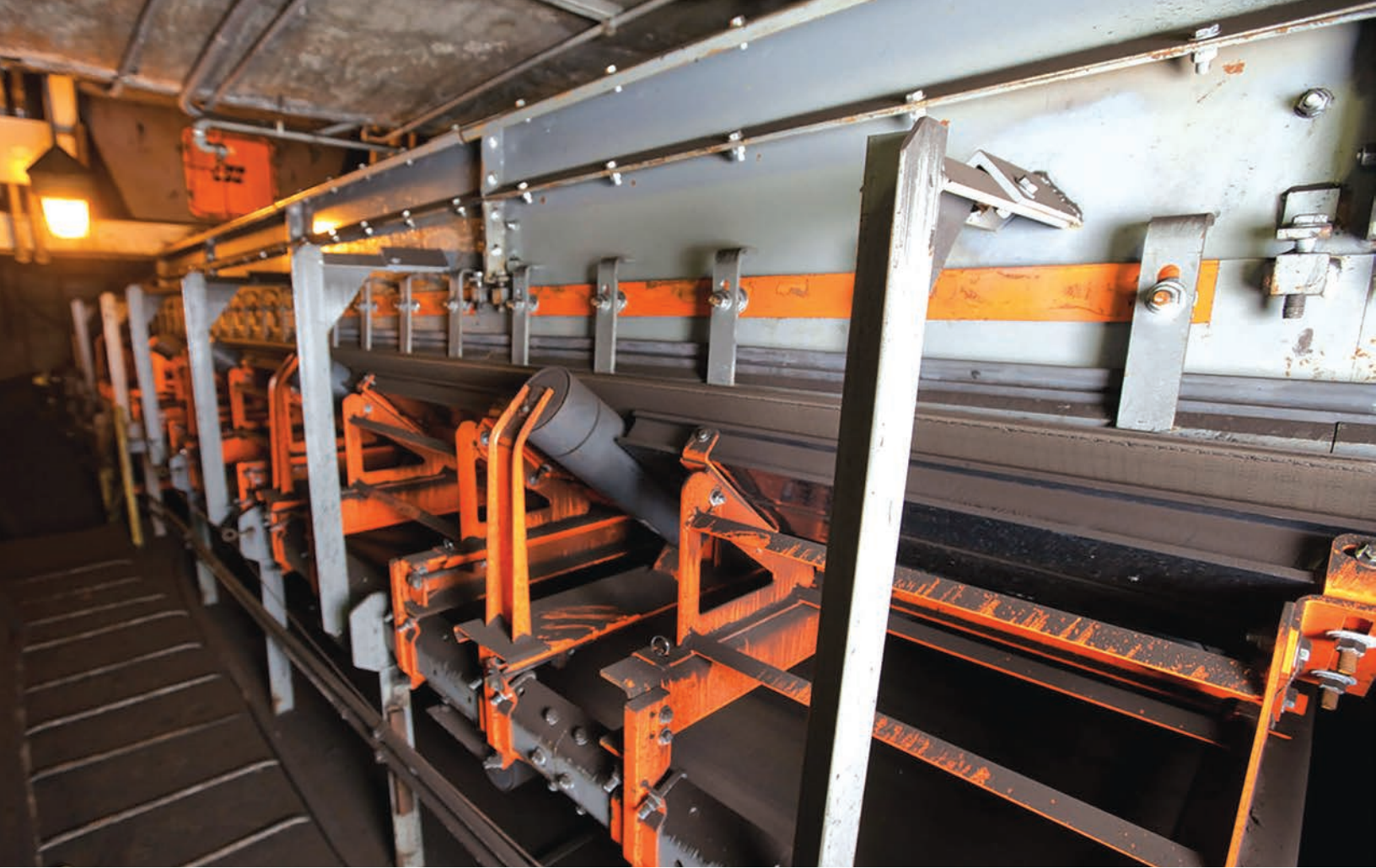
Inspection doors and track-mounted components facilitate maintenance for extended equipment life. PHOTO: MARTIN ENGINEERING
