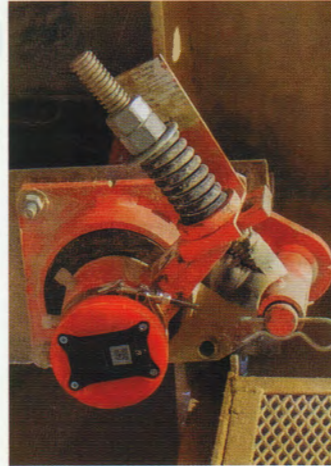
The Rotary Twist™ Tensioner with a Primary Cleaner helps retain a tight fit for the blade across the belt plane
