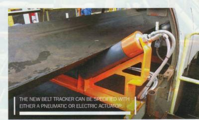
either to an electrical relay or a pneumatic solenoid to extend or retract the cylinder as needed, depending on which version is specified."
