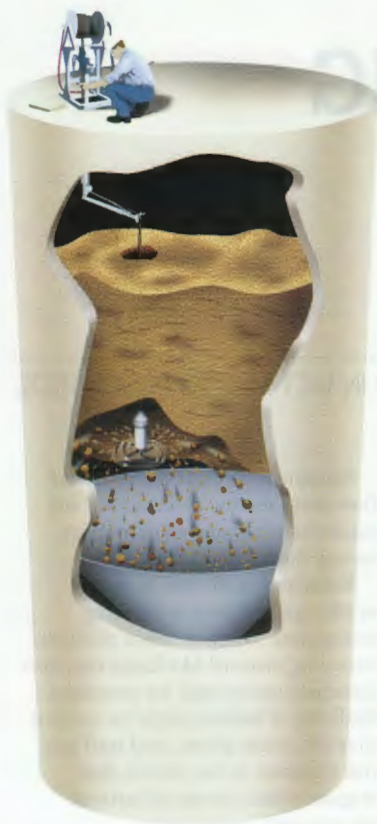
CLEANING REQUIRES TOOLS THAT WORK INSIDE THE SILO FROM THE TOP, CONTROLLED BY PERSONNEL OUTSIDE.
