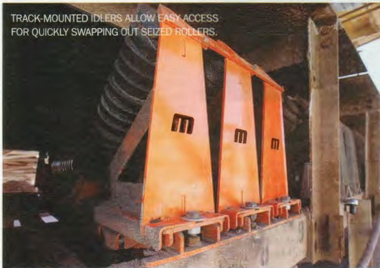
TRACK-MOUNTED DESIGNS ALLOW COMPONENTS TO SLIDE IN AND OUT EASILY FOR MAINTENANCE.
