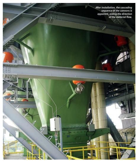
After evaluating the problem, Martin Engineering recommended the installation of 18 Martin Air Cannons. Fed by the compressed air system and discharged either on a schedule or manually from a convenient central location, air cannons provide effective performance by supplying a powerful discharge of air that dislodges material buildups and enhances the flow of bulk solids.
