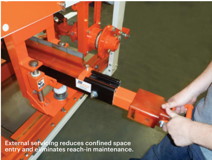
The slide-out design is engineered for safe access and replacement of the blade cartridge by a single worker.
