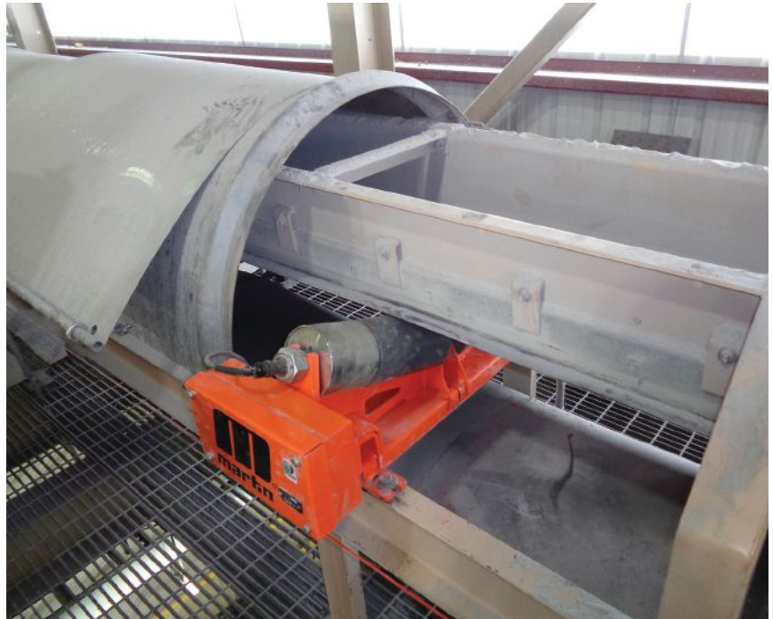
A single Roll Generator has enough power output to run a variety of accessories.
