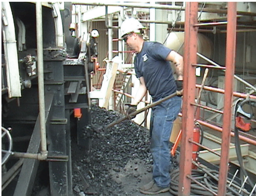
Cleaning up spillage exposes workers to a potential hazard area from the moving conveyor.
