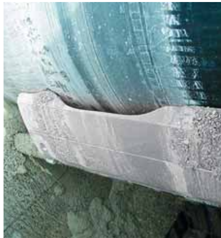
Wear to a conveyor belt cleaner blade can create a wear pattern known as a 'smiley face' or 'mooning'
