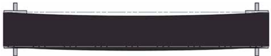
Figure 2 – A tracker pivots against the mistracking, using the force and weight of the belt to redirect it
