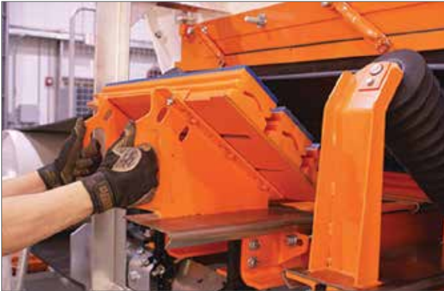
The track-mounted systems can be serviced quickly and safely, with no reach-in maintenance.
