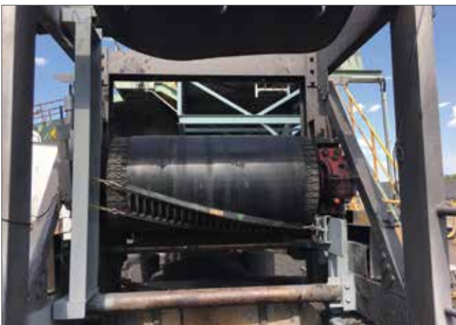
The unique belt cleaner forms a 3-D curve beneath the discharge that conforms to the pulley's shape.
