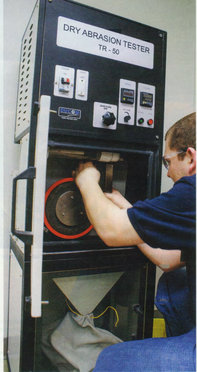
2 A dry abrasion tester checks three-body abrasive wear, such as between a conveyor belt, chute liner and bulk material
