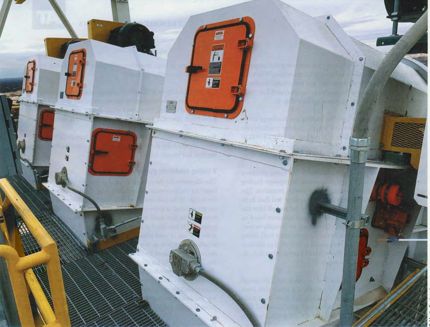
4 Strategically-located access doors facilitate inspection and service
