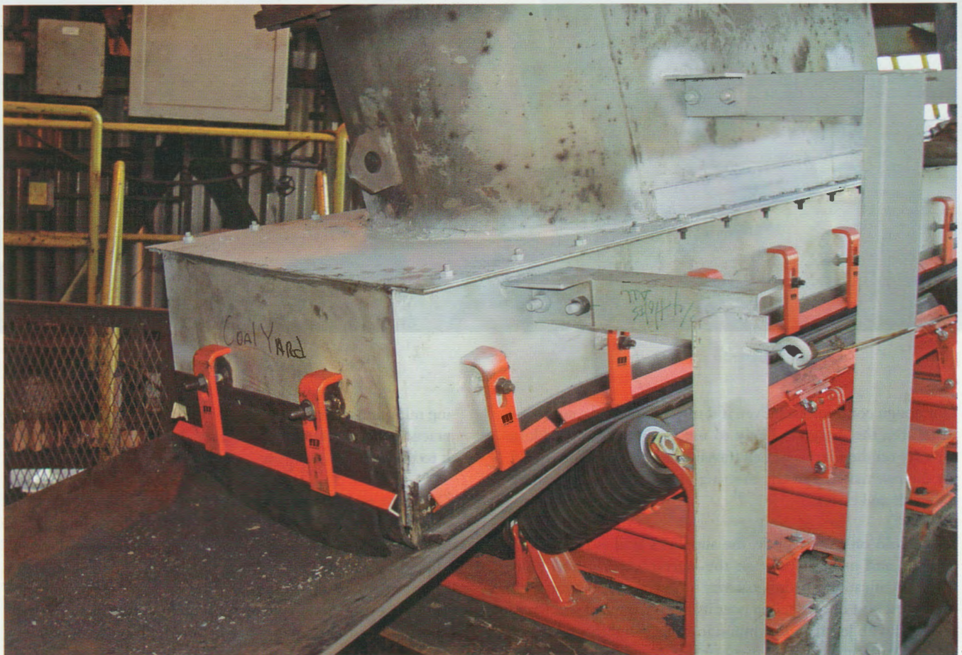
2 Curtains on the tail box can control the bouncing and rollback of round cargo
